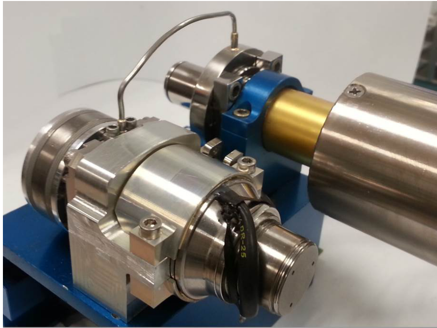
Figure 10. K527 cooler with K508 cold head
