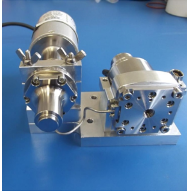
Figure 15. K527 rigid interfacing without TDA
